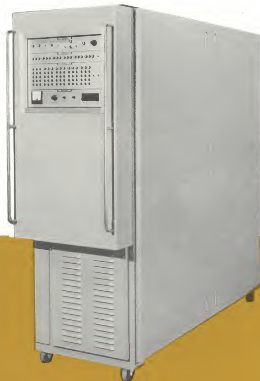
Series MT mass core memory. The first practical mass core memory to offer over 20-million bit capacity with economy.
